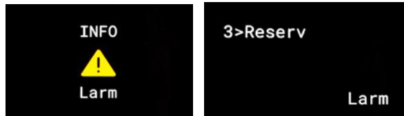
The first screen shows the alarm type, and the second shows the alarm source.
