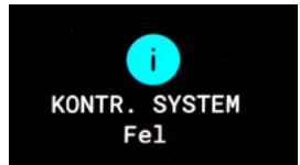
It is not possible to arm an area if certain system faults have occurred. These fault messages can be temporarily deactivated in the same way as active zones (see above). The alarm manager should inform users whether they have the authorization to deactivate fault messages in this way or not.
